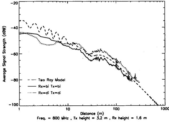
Fig. 2. Validation measurements for a rural LOS path.
