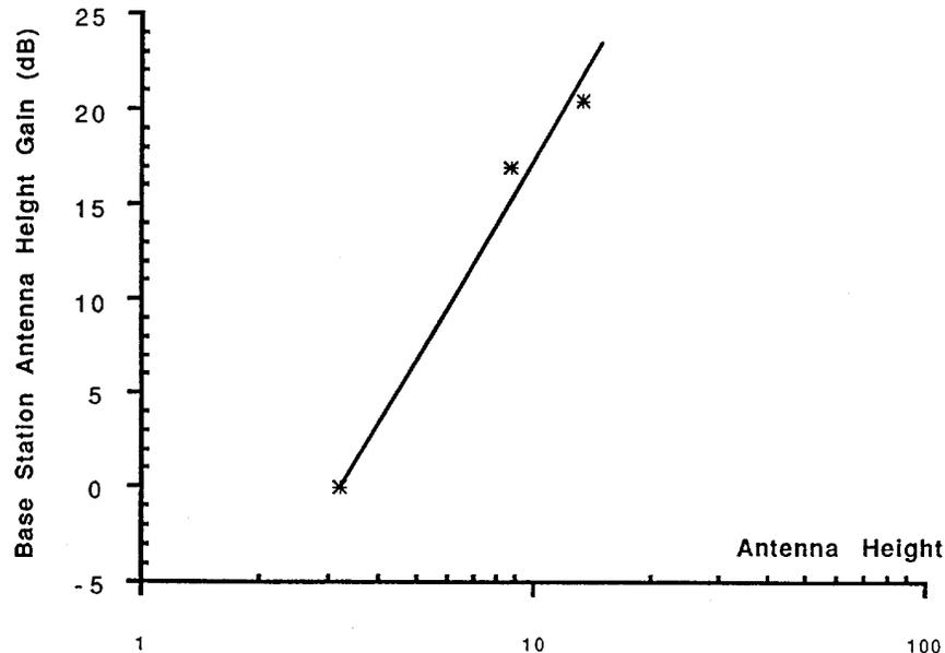
Fig. 10. Base station antenna height gain for a suburban LOS path in Mission, San Francisco.
