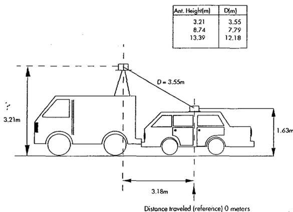
Fig. 1. Initial reference position for stationary transmitting van and mobile receiving van.
