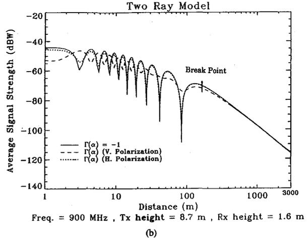
Fig. 3. Two-ray model showing: (a) the ray paths; and (b) the receiving power for vertical and horizontal polarization and assuming  $\Gamma = 1$ .
