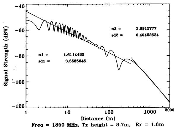
Fig. 4. Multiple slope regression fit to the two-ray model.
