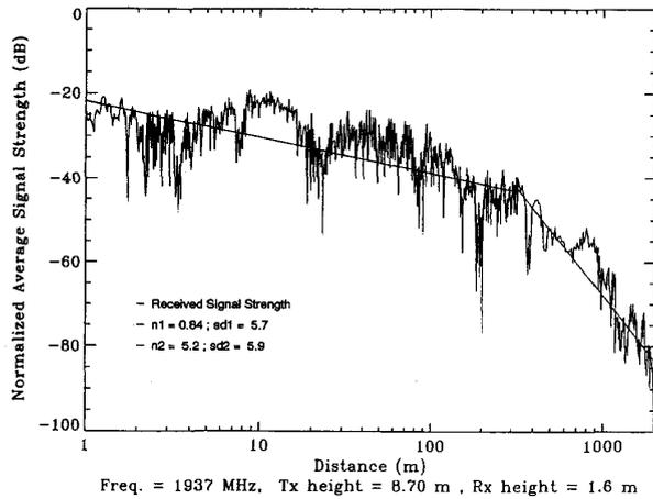
Fig. 6. Normalized composite signal curve for a suburban LOS path along Mission Street, San Francisco.
