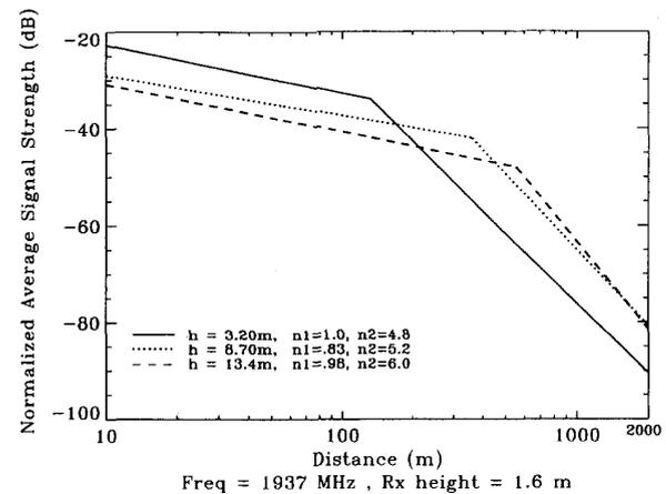
Fig. 9. Regression comparison for LOS measurements at three different antenna heights.
