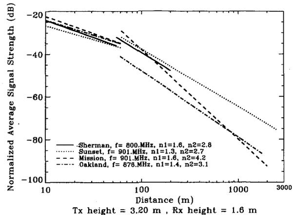
Fig. 8. Regression comparison for LOS measurements in different environments.
