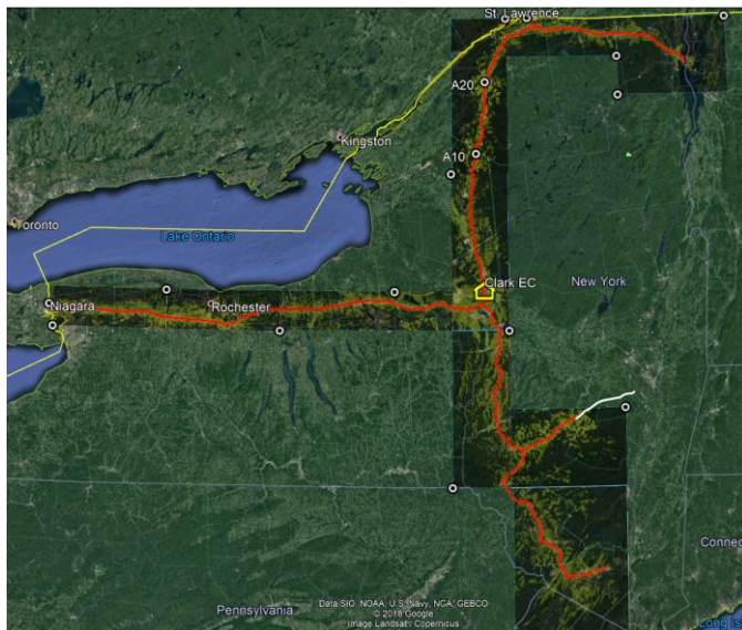
Fig. 7: End result of 46 Base Stations covering the Droneway in New York.
